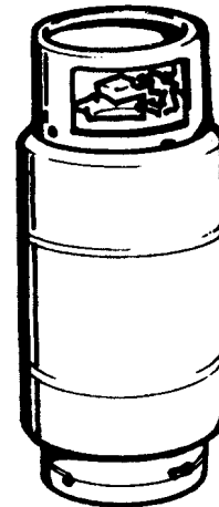
VAPOR WITHDRAWAL LP-GAS 250 LBS. PRESSURE
